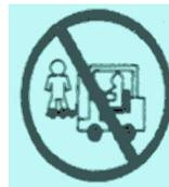
To insure personnel Safety, persons should not be on the pallet during transport/lifting the forklift.
