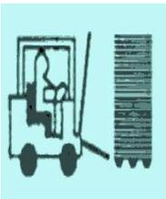
You can de-stack Presswood Pallets easily at any time. First tilt the Forklift Truck mast forwards, then enter the forks at the point of separation to lift the pallets.
